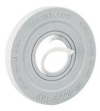
The single membrane rings are peeled off according to the diameter of the routed cable/hose. For this purpose, only a small hole between the rings needs to be pierced. Then the corresponding ring can be removed.
