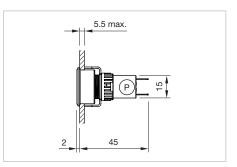
Dimensions [mm] P = Plug-in terminal 2.8 x 0.5 mm
